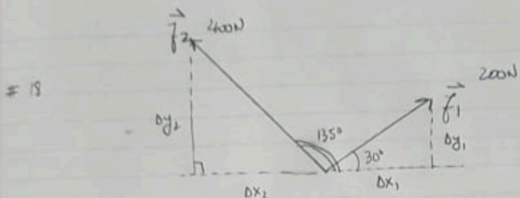
$$\vec{f}_1: \Delta x_1 = 200 \cos 30^\circ = 173,21 \quad \left. \begin{array}{l} \vec{f}_2: \Delta x_2 = 400 \cos 135^\circ = -282,84 \\ \Delta y_1 = 200 \sin 30^\circ = 100 \quad \Delta y_2 = 400 \sin 135^\circ = 282,84 \end{array} \right\}$$
